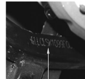
The frame number is stamped on the frame between the front wheels.
